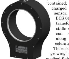
charged particle beam sensor. The licensed BCS-01 is a DC current transformer that installs over a commercial vacuum break along the particle accelerator beamline. There is a very large and growing demand in the medical field for beam ther-
