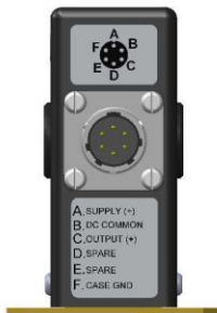
CONNECTOR OPTION ADD "-C" TO PART NO. CONNECTOR PART NO. PT023-10-6P-023 PT02E-10-6P OR EQUIV. MATING CONNECTOR PT06A-10-6S-023 OR PT06A-10-6S OR EQUIV.
